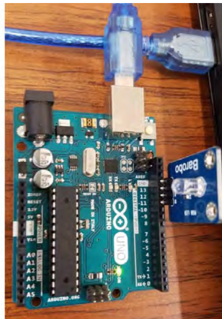
Figure 7.10: Connecting the Arduino to the Computer via USB cable (only the two ends of the blue USB cable are shown—it’s all one cable)
